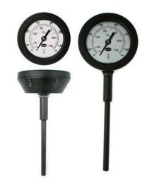
The 93 marine exhaust gas pyrometers are specially designed to measure the temperature of engine exhaust gas. These instruments are robust enough to withstand the vibrations, temperatures and the environment of a diesel engine.
