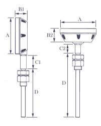
93 Marine Exhaust Gas Pyrometer
