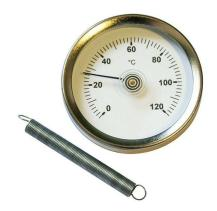
The JV210012 is a bi-metal temperature gauge which is used to measure the surface temperature of pipework by use of a spring around the pipe, the maximum diameter of pipework is 25mm.
