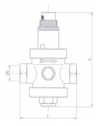
The JV141002 is an economical WRAS approved pressure reducing valve which is suitable for water up to 80°C, Used in domestic water supply systems as well as commercial and industrial plants, this is a versatile valve suitable for many duties.
