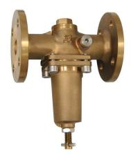
The JV140021 is an accurate and reliable direct acting pressure reducing valve used to maintain a pre-set downstream pressure regardless of flow rate and upstream pressure fluctuations. It is particularly suitable where a positive shut-off is required under "no flow" conditions.
