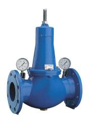
The JV140019 is an accurate and reliable direct acting pressure reducing valve used to maintain a pre-set downstream pressure regardless of flow rate and upstream pressure fluctuations.
