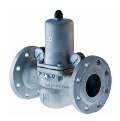
The 482 is an extremely sturdy pressure reducing valve which is suitable for water up to 95°C, compressed air, neutral gas, neutral and non-sticking liquids. Used in domestic water supply systems as well as commercial and industrial plants, this is a versatile valve suitable for many duties.
