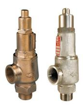
The 480/485/490 are suitable for use with positive displacement pumps either of the rotary or reciprocating type and have been used successfully with water and most corrosive liquids. They can also be used as a relief or combined relief and bypass valve and can be modified to operate as an integral pump by-pass relief valve.
