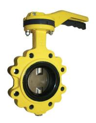
BSI gas approved butterfly valve with a NBR liner, lugged and tapped to PN16.
