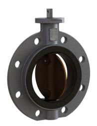
Marine quality butterfly valve with a bonded NBR liner suitable for many duties including oils and hydrocarbons.
