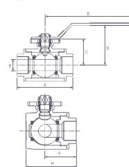
A three-way, L-Ported stainless steel ball valve making them suitable for many applications where fluid diversion is required.
