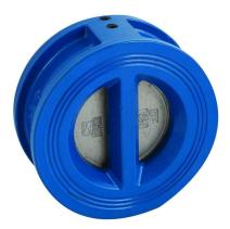
The JV081016 is an epoxy coated cast iron, spring loaded dual plate check valve with stainless steel flaps and EPDM seats suitable for water applications.
