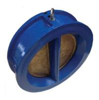
The JV081015 is an ANSI 150 cast iron, spring loaded dual plate check valve with stainless steel flaps and NBR seats suitable for various applications.
