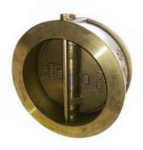
A marine duty ali-bronze, spring loaded dual plate check valve with ali-bronze flaps and NBR seats suitable for cold and hot water, seawater, fuel oil and other non-aggressive medium.
