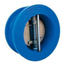
A WRAS approved epoxy coated cast iron, spring loaded dual plate check valve with stainless steel flaps and EPDM seats suitable for water applications.
