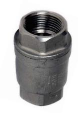
The JV081001 is a good quality stainless steel spring loaded check (non-return) valve. This valve requires a minimum pressure of 0.04 bar to open and can be installed in both horizontal and vertical lines with upward flow or in any intermediate position.
