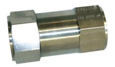
A high pressure spring-loaded non-return valve with a stainless steel body and Buna-N seals. The valve requires a minimum pressure of 0.33 PSI to open and can be installed in both horizontal and vertical lines with upward flow or in any intermediate position.
