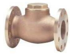
A bronze lift type check (non-return) valve with a bronze disc conforming JIS Japanese specifications. It must be fitted in the horizontal position.
