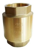
An economical spring-loaded non-return valve with a brass body and disc with Viton seals. The valve requires a low minimum pressure of 0.02 bar to open and can be installed in both horizontal and vertical lines with upward flow or in any intermediate position.
