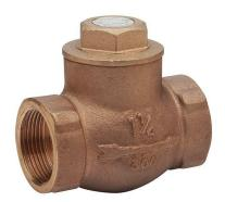
An economical bronze swing type check (nonreturn) valve with low cracking pressures. Can be installed in horizontal and vertical lines with upward flow.
