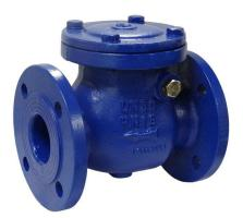
A robust swing type (flapper) check valve with an iron disc and bronze trim suitable for cold and hot water, fuel oil and other non-aggressive medium.
