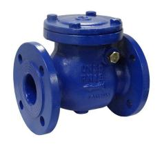
A robust ductile iron, swing type (flapper) check valve with a ductile iron disc and NBR seals suitable for cold and hot water, seawater, fuel oil and other non-aggressive medium.
