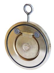
A marine quality aluminium bronze spring Approvals, Features & Benefits loaded flap type check (non-return) valve used to prevent backflow in water and • seawater systems and can be used in other  $\bullet$ applications providing the valve materials are compatible with the media.
