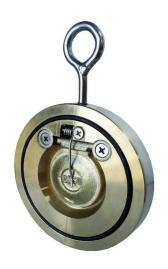
A marine quality aluminium bronze spring loaded flap type check (non-return) valve used to prevent backflow in water and seawater systems and can be used in other applications providing the valve materials are compatible with the media.
