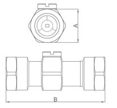
JV080008 Floguard ® DZR Brass Body EPDM Seal Spring-Loaded
