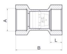
JV080007 <sup>38 Series</sup> DZR Brass Body EPDM Seal Spring-Loaded Check (Non-Return) Valve BSPP Threaded
