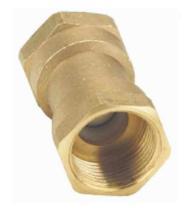
A WRAS approved economical spring-loaded non-return valve with a DZR brass body and EPDM seals. The valve requires a minimum pressure of 0.1 bar to open and can be installed in both horizontal and vertical lines with upward flow or in any intermediate position.
