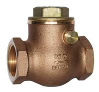
This bronze swing type check valves is suited for steam, water and oil applications. It can be fitted in the horizontal position or in the vertical position with the flow going upwards. This valve requires a low minimum pressure to open.
