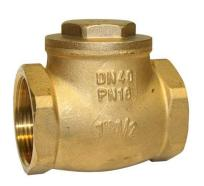
An economical swing type check (non-return) valve with a brass body and NBR seals. Can be installed in horizontal and vertical lines with upward flow.
