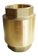
An economical spring-loaded non-return valve with a brass body and NBR seals. The valve requires a low minimum pressure of 0.02 bar to open and can be installed in both horizontal and vertical lines with upward flow or in any intermediate position.
